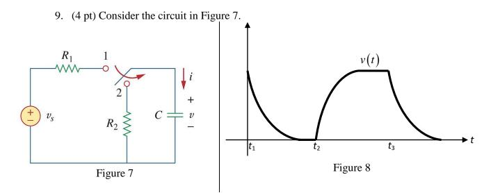
Assume that the switch has been in position 1 during time t < 0. Then, during time  $t \ge 0$  the switch changes its position three times: at  $t_1$ ,  $t_2$ ,  $t_3$ . (At time  $t_1$ , the switch changes to position 2. At time  $t_2$ , the switch changes back to position 1. At time  $t_3$ , the switch changes again to position 2.)
